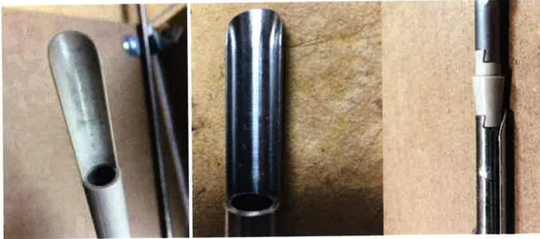
Figure 22: All parts were again visually inspected for wear and structural damage. Scuff marks and discoloration can be seen on the inner diameters of the peek and stainless steel follower sleeve tongues. Although not clearly visible from the available pictures, slight discoloration was also present on the peek conical bearing displayed on the right.
