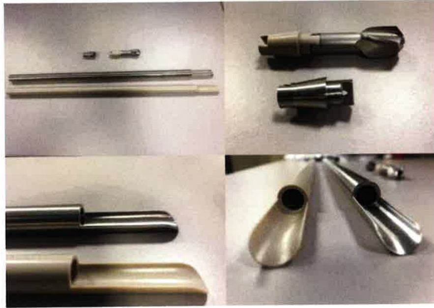
Figure 10: the two follower sleeves and conical inserts are shown above. Experimentation has shown that deflected reaming has no damaging effects on either the peek or the stainless steel parts.
